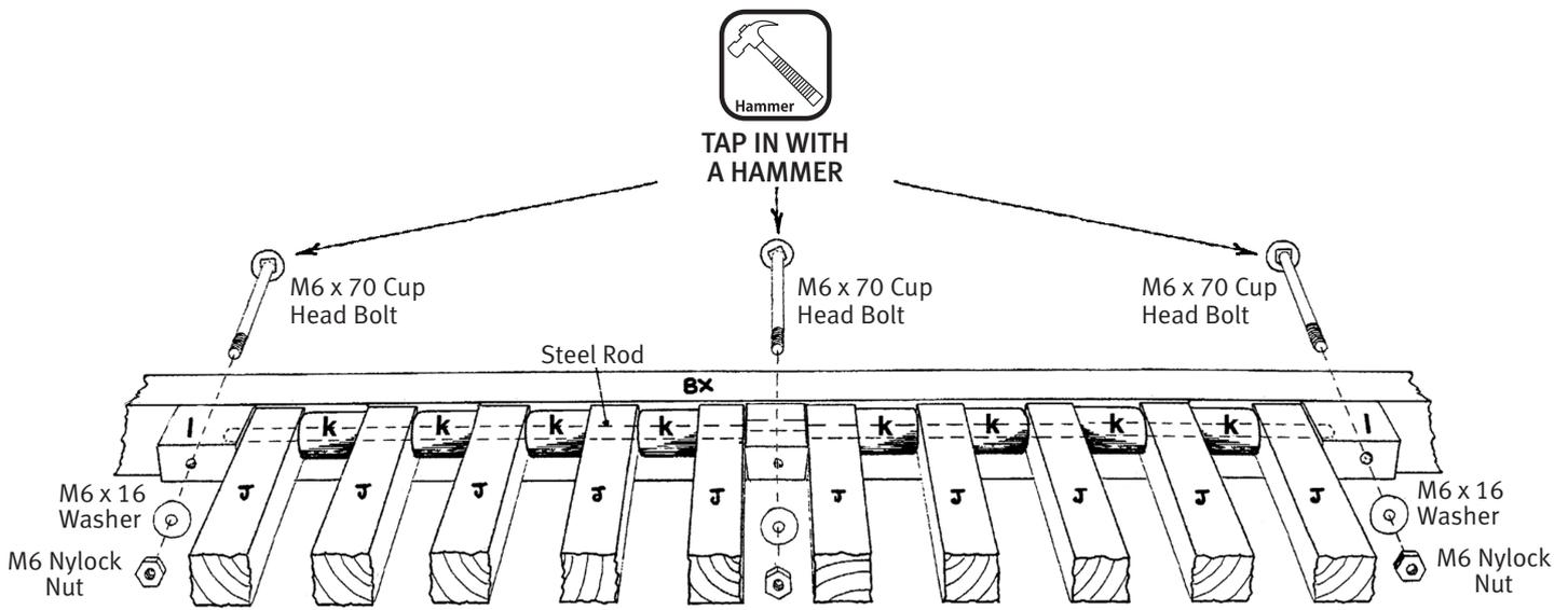
14. Slide 5 treadles J onto the steel treadle rod with a round wooden spacers k between. Add the centre block. Then add the next 5 treadles and round wooden spacers followed by the treadle blocks l at either end. Note that the rod holes in the treadle blocks must be towards the top. Then bolt all 3 blocks to BX with M6 x 70 Cup Head Bolt, M6 X 16 Washer, and M6 Nylock Nut. Tap the head into the wood with a hammer.
