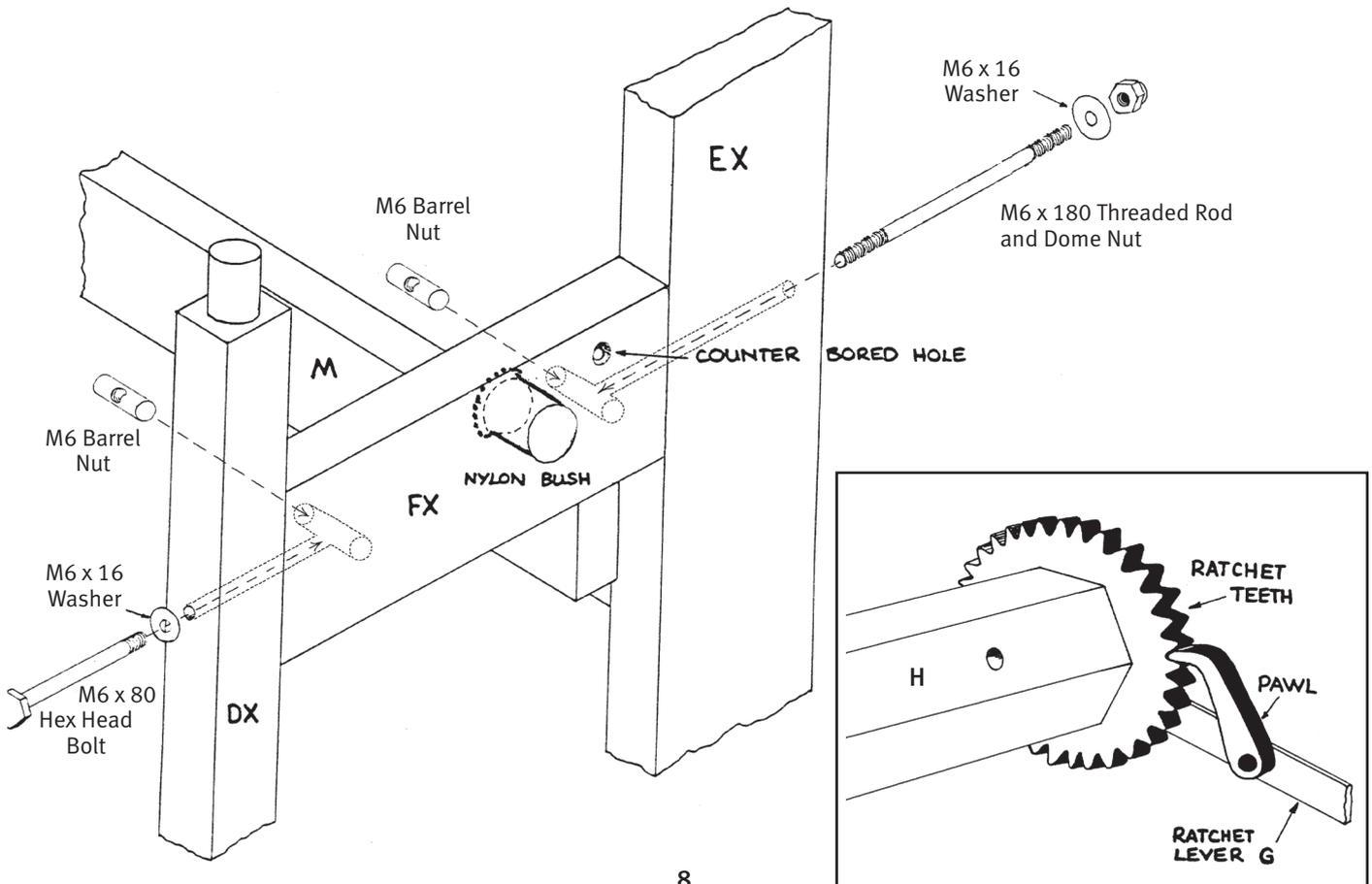
12. Insert the 12 x 1 Pan Head Screw into the inside of the front upright DX for a ratchet lever stop. When transporting the loom lift and pull the lever sideways, then let it hang down.
