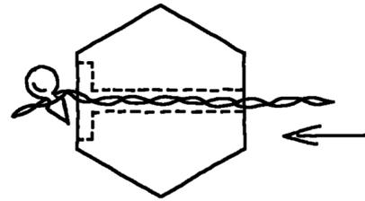
Use the third warp stick for your end warp stick (refer to warp instructions) and attach to the end of the Texsolv cord with a Texsolv peg through the 6th hole.
