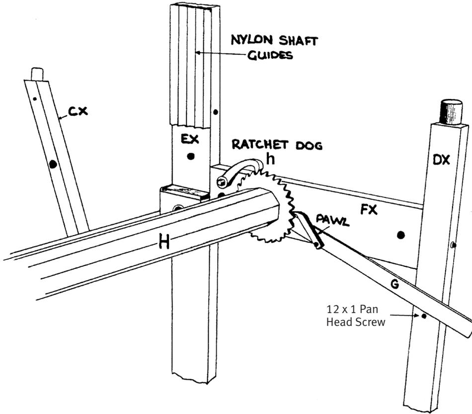
13. Attach the ratchet dog to the right cloth beam support FX using a M8 x 50 Hex Head Bolt, M10 Hex Nut, M8 x 19 Washer and M8 Nylock Nut. Tap the head of the bolt into the counter-bored hole. Do not overtighten as the dog should move freely after tightening the nut.
