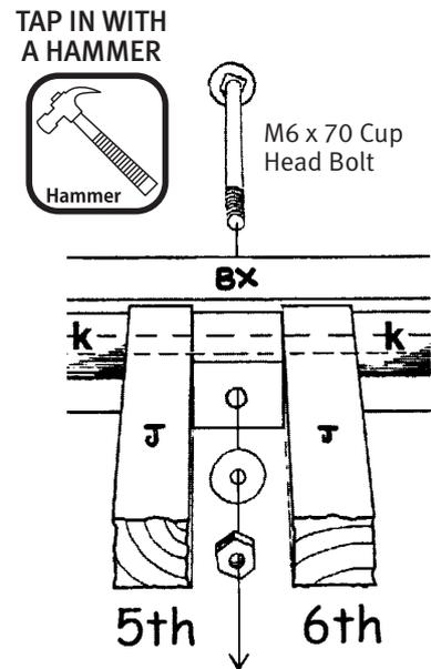
15. Push a M6 x 50 Cup Head Bolt through the inside of back upright CX and tap the head of the bolt into the wood with a hammer. Then attach spacer P through the hole with a M6 x 22 Washer and nylon knob.
