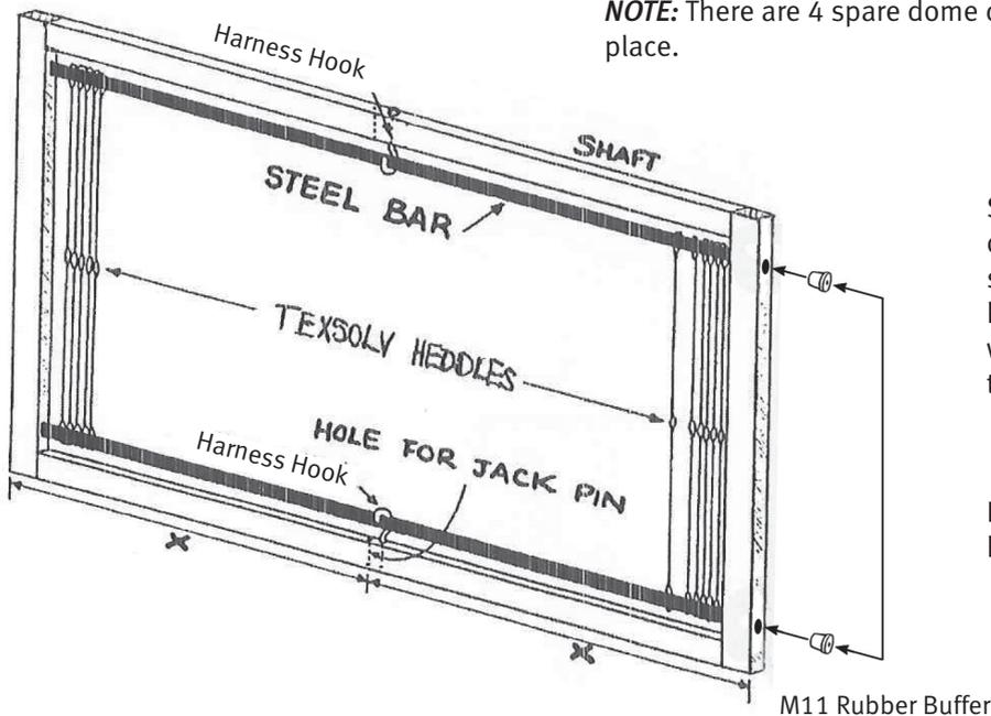
Spread the heddles evenly either side of the Harness Hook and then clip the stainless steel rods over the hooks. The hooks prevent the bars from sagging when being raised or pulling out when the warp is being advanced.
