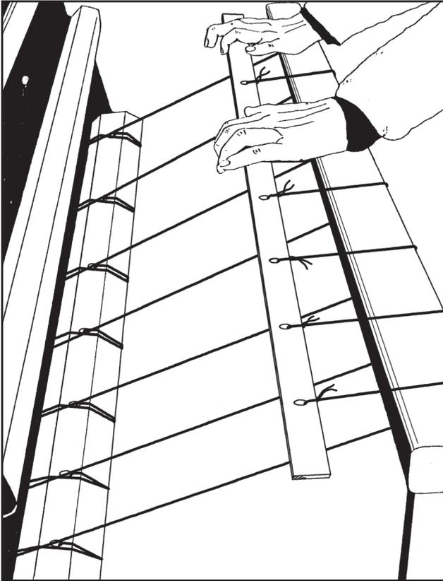
To attach a warp stick to the front roller, thread 1 Texsolv cord through the first hole in the warp stick and back through the second to end hole in the cord.
